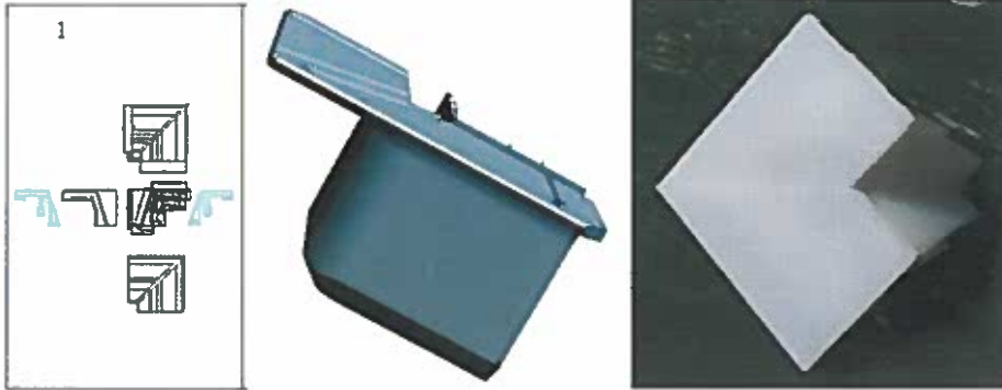
Drawing, 3D model and printed 3D prototype of a corner profile
